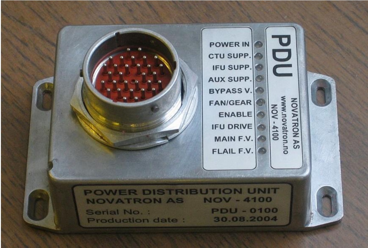
Picture 4: Power Distribution Unit
