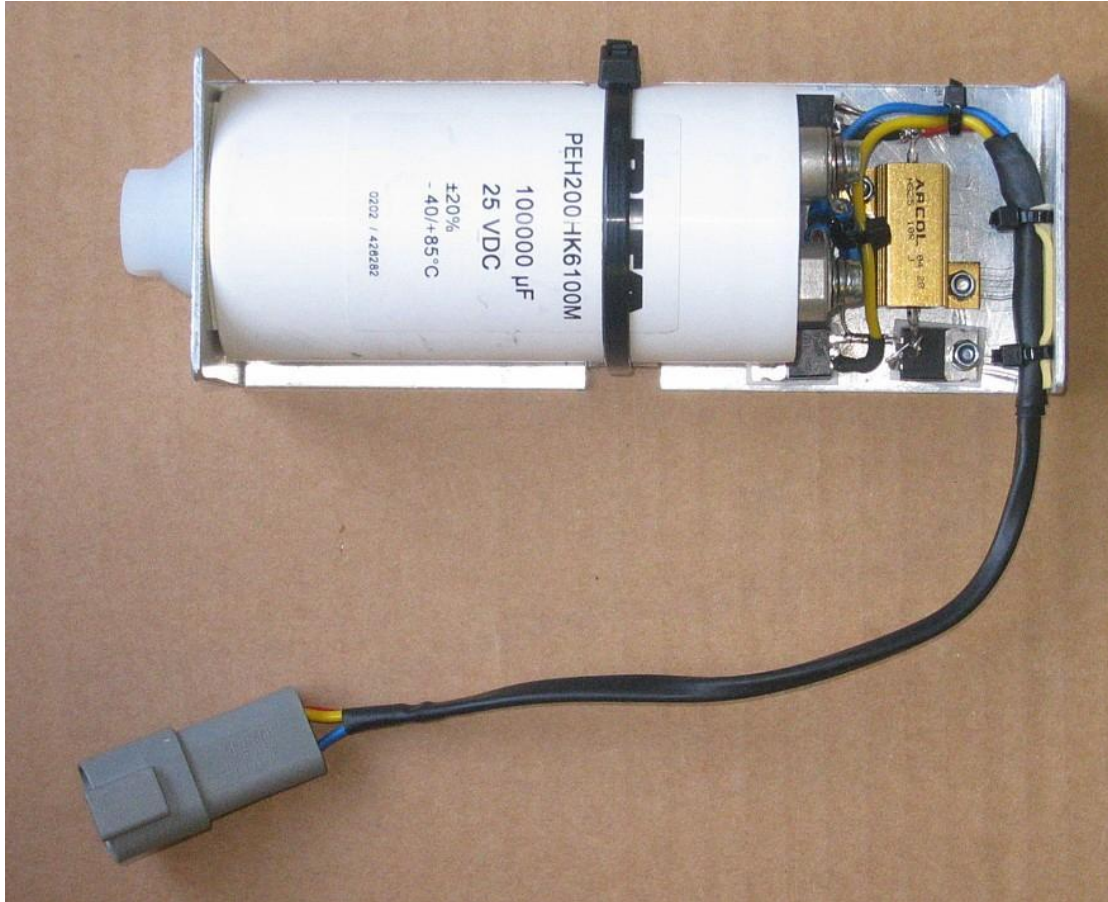
Picture 7: Voltage stabilizer module
