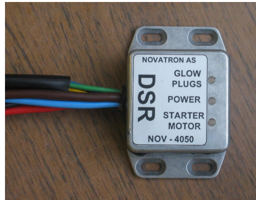
Picture 6: DSR - Dual Smart Relay
